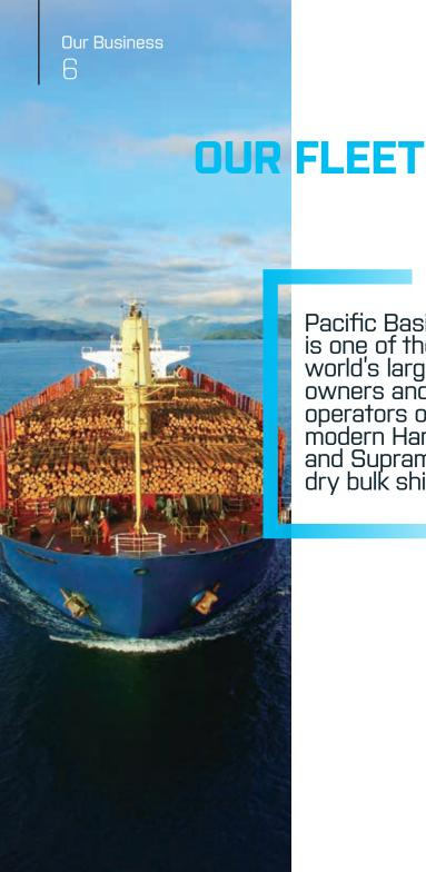
Pacific Basin is one of the world's largest owners and operators of modern Handysize and Supramax dry bulk ships Our geared bulk carriers are highly versatile self-loading and self-discharging ships
