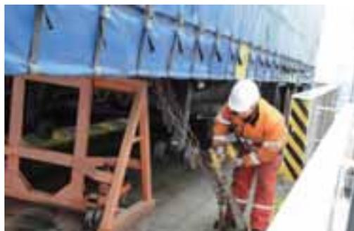
Trailers being secured in preparation for sailing
